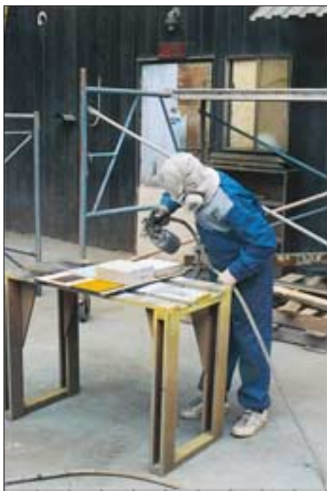
Fig. 2 - Spray application of coatings for testing Photos and figures courtesy of the authors
