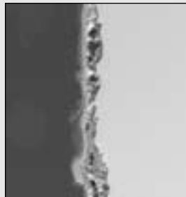
Fig 7D - Coating D on rust — no penetration
