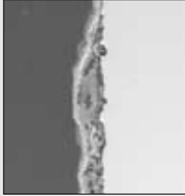
Fig 7B - Coating B on rust penetrates rust and interface
