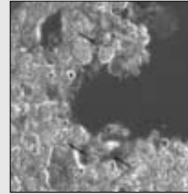
Fig 4 - Penetration of coating A into fine porosity of the surface
