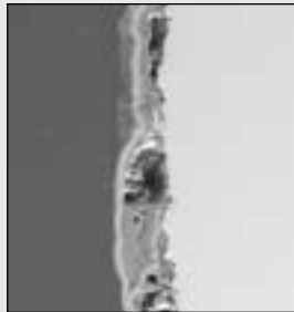
Fig 7C - Coating C on rust — no penetration
